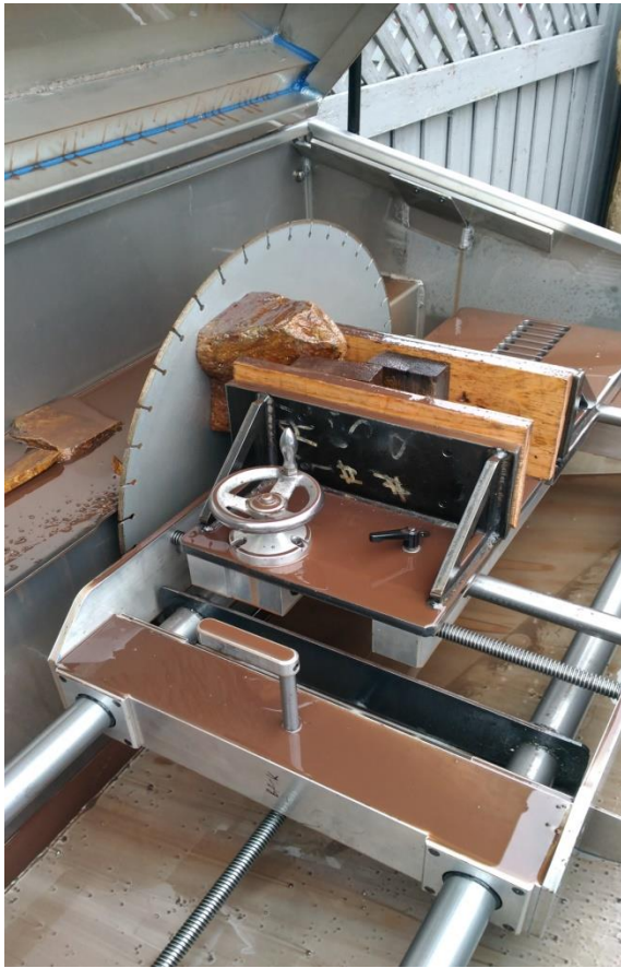
Cutting table has hand controls. narrow oil reservoir and sloped tray to feed coolant back into reservoir
