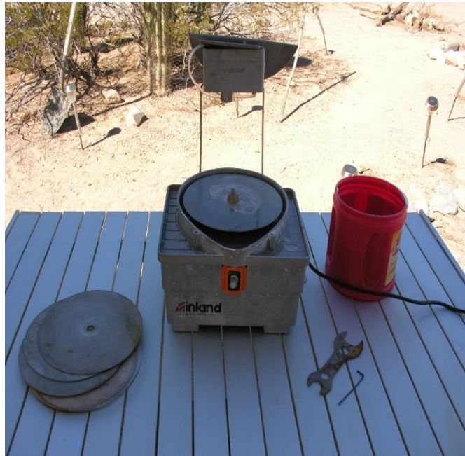
8" swaptop flatlapper, diamond grinding plates, water bucket and tools
