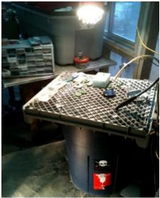
Carving jade generally requires the use of water to lubricate the cutting action of the diamonds in your tool bit as they grind against the surface of the stone. If you do not, and at the high speeds that's these burrs and wheels are spinning the friction will create a lot of heat and the metal bonding agents that hold the diamonds to your tool expand to much, and can allows the diamonds to fall out of your tool shortening its life and the cutting effect.
