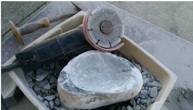
Using the angle grinder to cut out bowl shape
