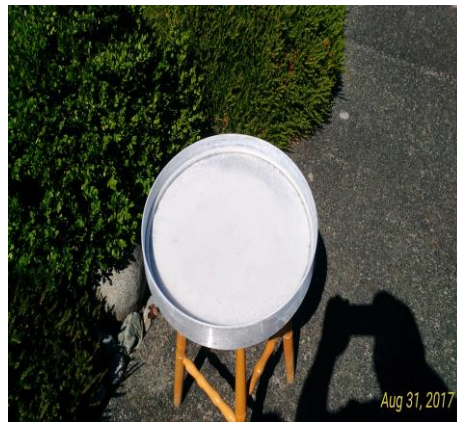
Dedicated polishing tray charged with tin oxide
