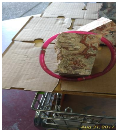
Protective tubing around rock
